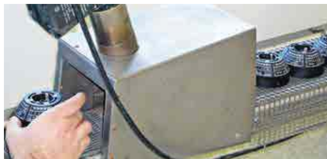
The HOTWIND is perfectly suited for drying and baking of print on plastic components.
