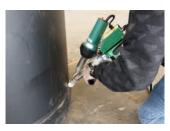
Welding is easily possible in tight spaces. The powerful motor and the few electronic components make the extruder fail-proof and durable.
