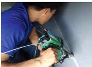
Welding is easily possible in tight spaces. The powerful motor and the few electronic components make the extruder fail-proof and durable.
