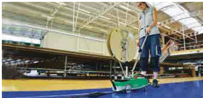
An economical, ergonomic tool for welding reinforcement tapes.
